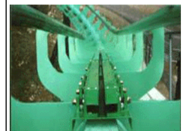
Figure 2. (a-top) Magnetic brakes installed in 2002 on the Jack Rabbit . (b-bottom) Magnetic brakes also were installed in Kennywood's newest coaster.
